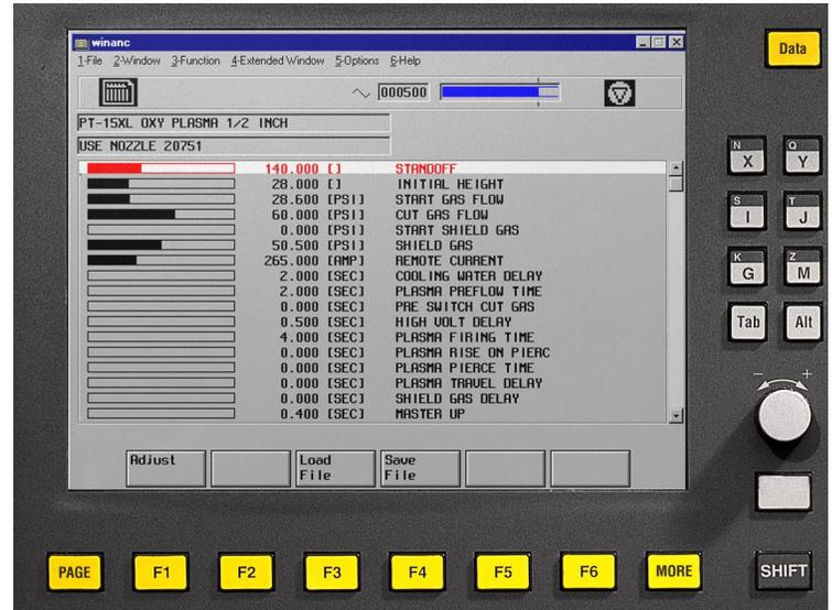
All process parameters are set automatically when a parameter set (SDP File) is selected. The operator can make adjustments on screen, at the CNC. Simply turn the handwheel to adjust each value. A graphical bar indicates each parameter's setting.
